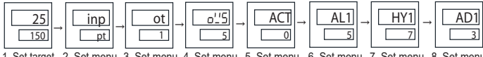
1. Set target temperature SV=150 2. Set menu INP=pt 3. Set menu OT=1 4. Set menu OVS=5 5. Set menu ACT=0 6. Set menu AL1=5 7. Set menu HY1=7 8. Set menu AD1=3
