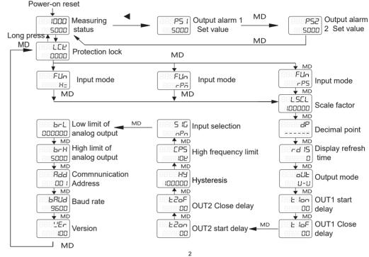
Figure A: Logic diagram of measured value and output alarm mode
