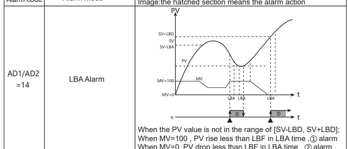
When the PV value is not in the range of [SV-LBD, SV+LBD]; When MV=100 , PV rise less than LBF in LBA time ,① alarm When MV=0, PV drop less than LBF in LBA time ,② alarm
